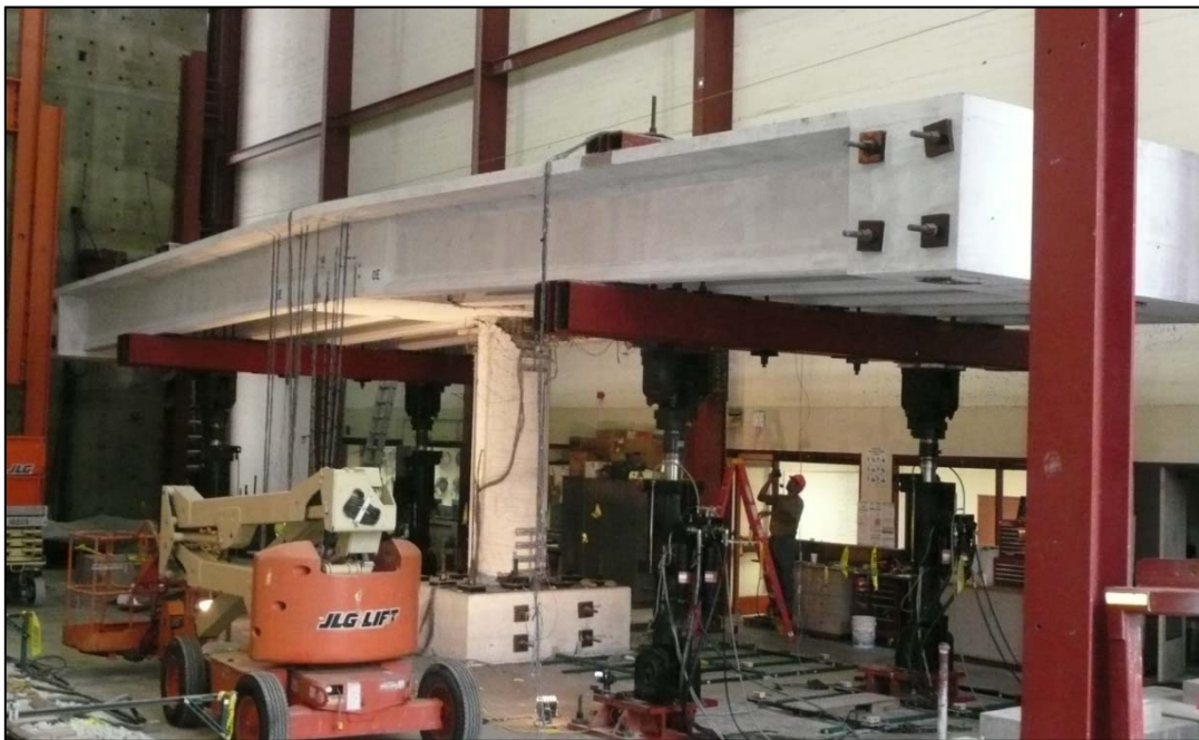
Figure 6.36: Displaced Test Unit at -6 in. of Displacement
