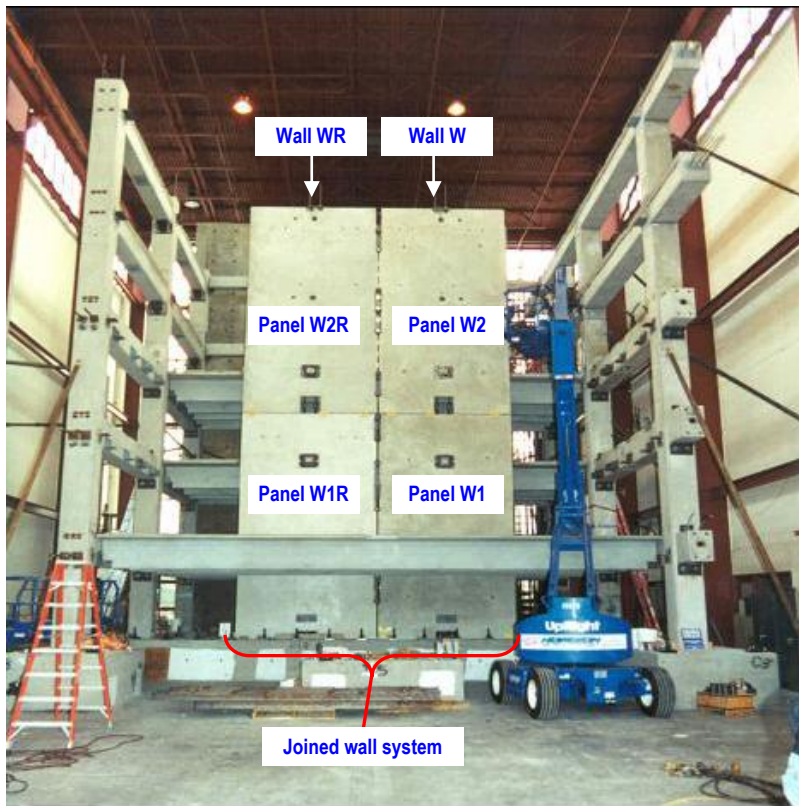
Figure 1.5 The two-wall jointed system included in the PRESSS building.
