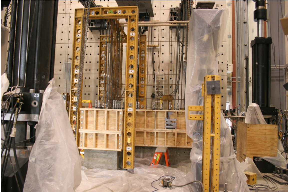
Figure 6.2 Two-part Base Block used for NTW2 to Expedite Construction
