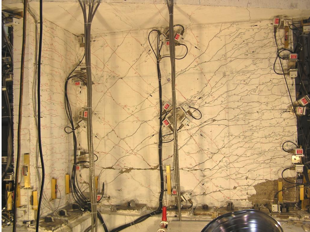
Figure 5.22 Observed cracking of NTW1 in the web
