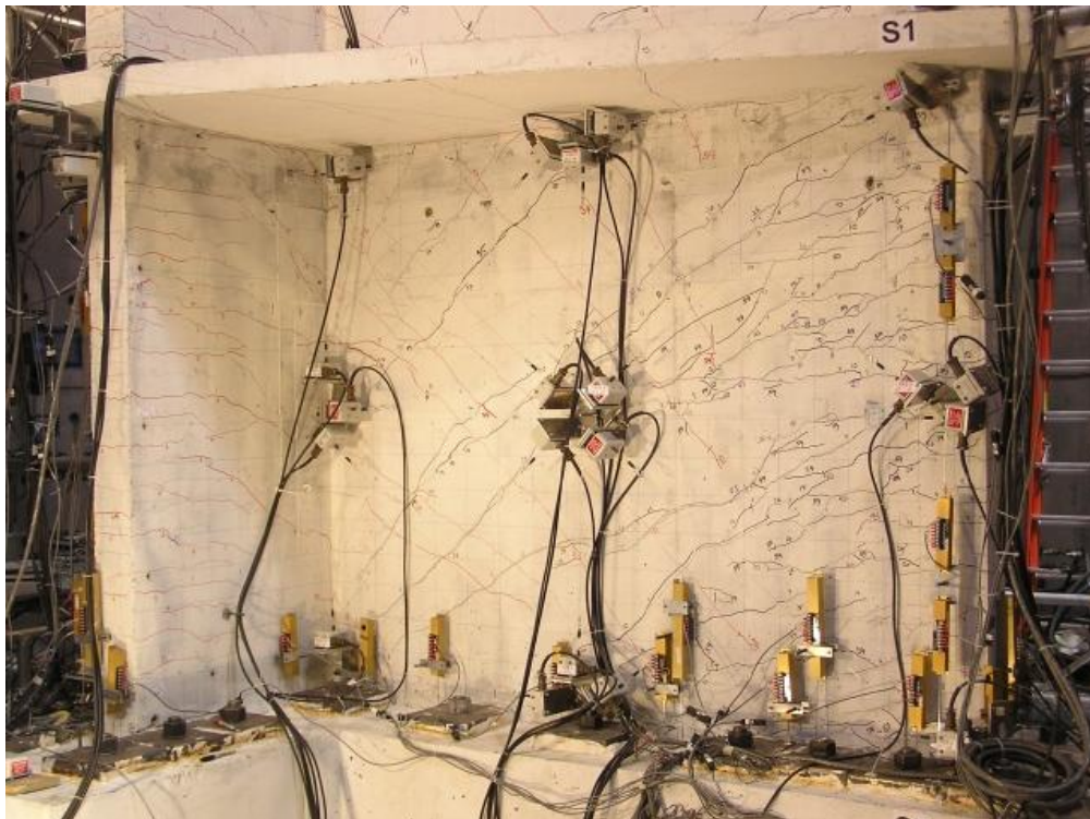
Figure 5.44 Condition of Web at First Floor After Subjected to 1% Drift Cycles
