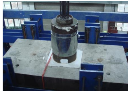
b) Post-tensioning anchor of the wall panel
