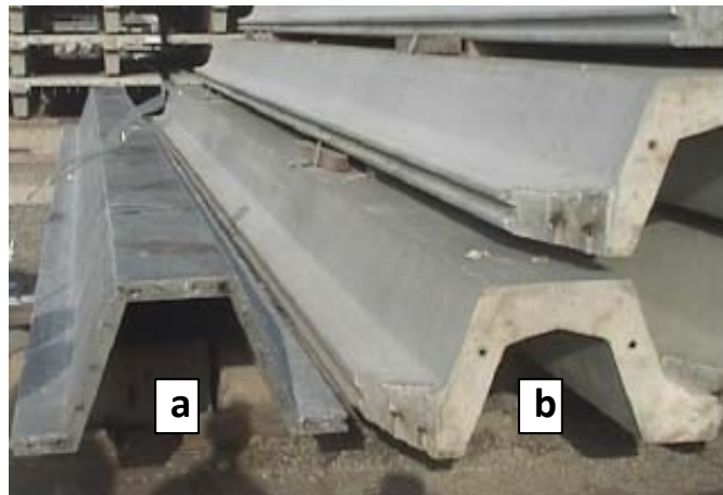
Figure 2.43. Comparison of a) SCFRC and b) conventional concrete sheet piles (Grünwald 2004)
