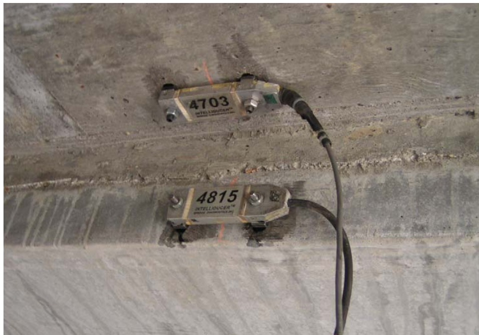
Figure 4.25. BDI strain transducers attached to concrete.
