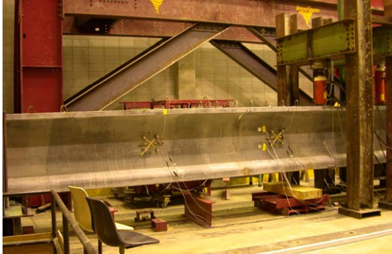
Figure 4.13. Large-scale flexure-shear test setup photograph.
