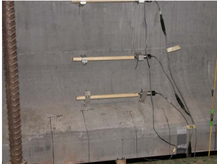
Figure 6.2. Flexural cracks on north bottom flange at midspan at peak load of large-scale flexure test.
