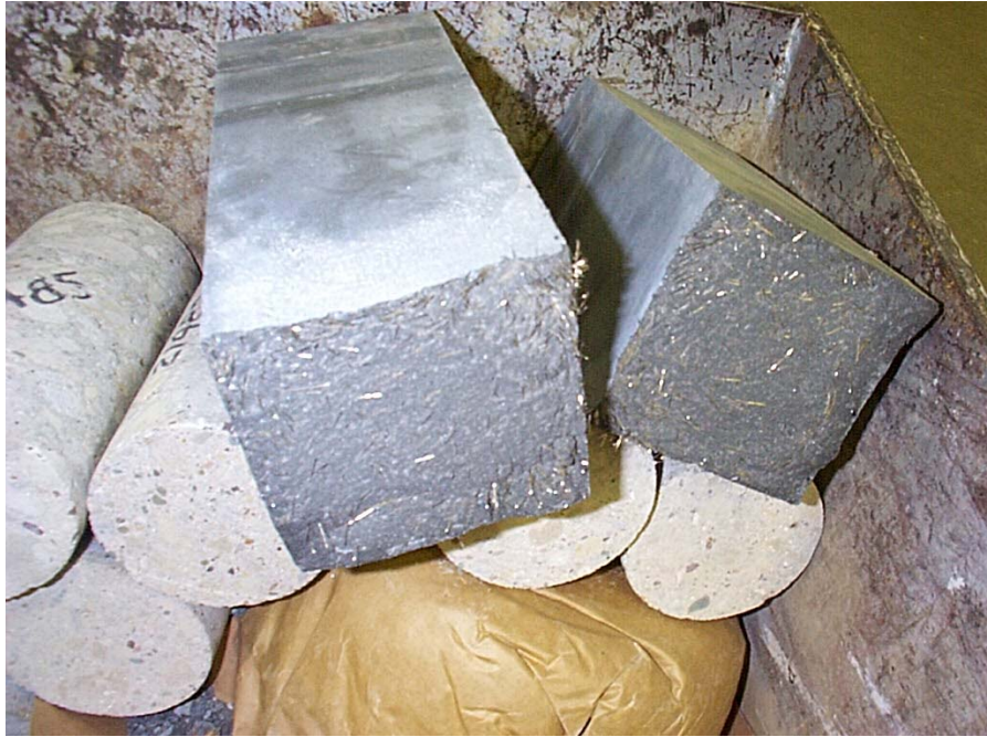
Figure 1.2. Samples of UHPC and conventional concrete.
